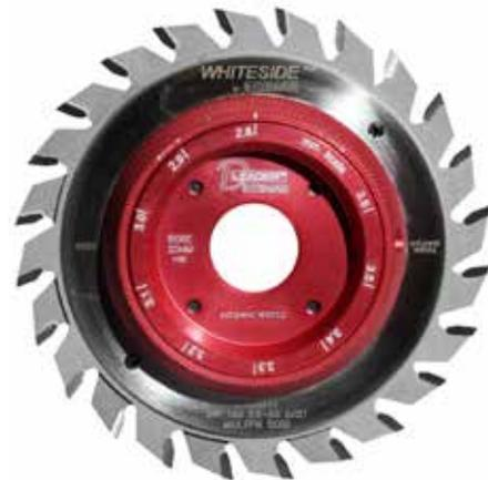
This scoring set eliminates the need for spacers, measuring, reassembling, testing, or adjusting that comes with traditional scoring blades. Simply loosen the locking screw and turn the dial to easily change the blade width from 2.8mm to 3.6mm. Bushings are included so that this set is compatible with 20mm, 22mm, or 3/4" shafts.
