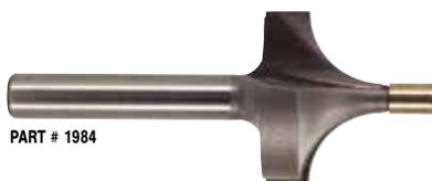
Extra small brass pilot (5/32" dia.) allows these bits to roundover edges on finely detailed workpieces with intricate contours, tight confines, and narrow openings. These bits give professional results without all the tedious hand sanding. Carbide cutting edges far outlast comparable high speed steel bits.
